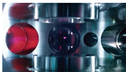
Figure 24: View through one of the viewports into the UHV chamber, where due to fluorescence light about 50 million cold Cs atoms can be seen as a small pink ball.
