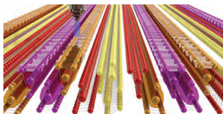
Figure 23: Charge density wave and atomic structure of NbS 3 -II polymorph.
